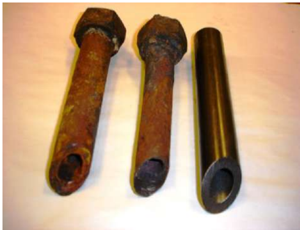
Figure 7. Treated – Baseline – Unused Coupons
