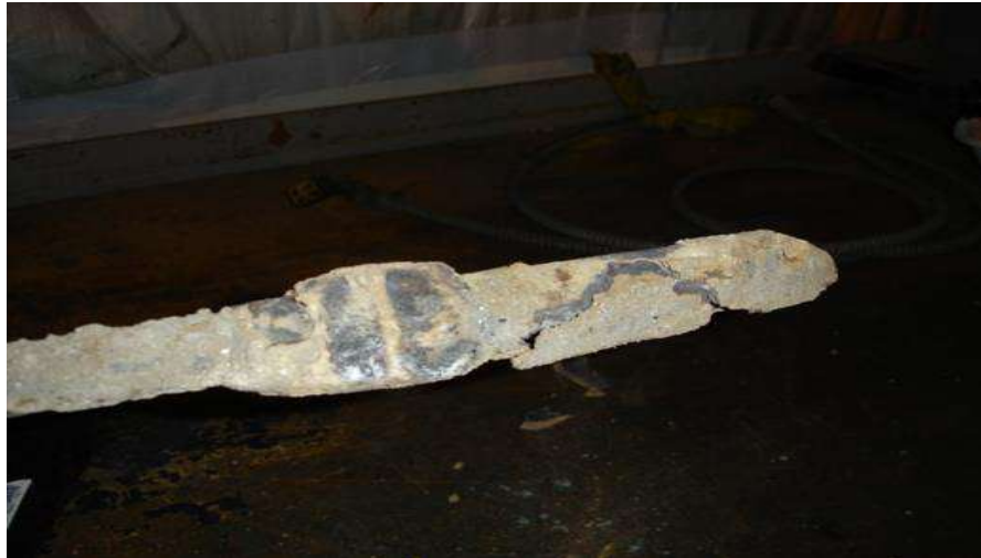
Figure 4. Corrosion Probe with Coupon and Slag Deposition.
