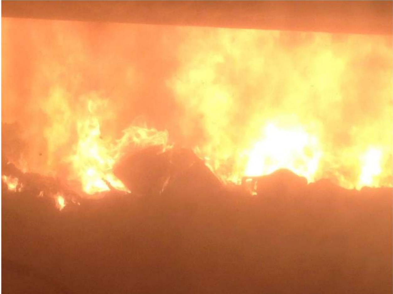
Figure 6 Image of the highly non-uniform combustion on an incinerator grate
