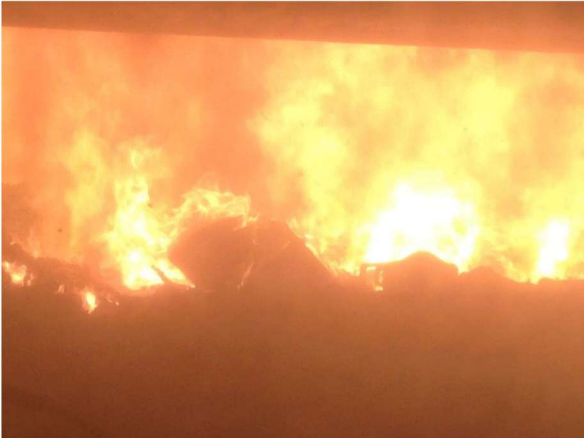
Figure 4 Image of the highly non-uniform combustion on an incinerator grate
